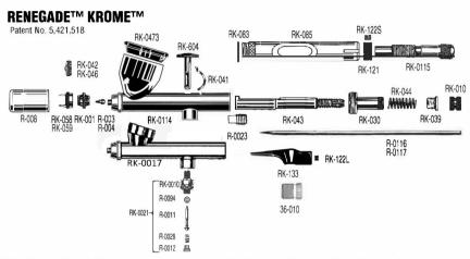
NOTE: Attached nozzle/tip housing has been permanently affixed to airbrush shell and is not made to be removed.
